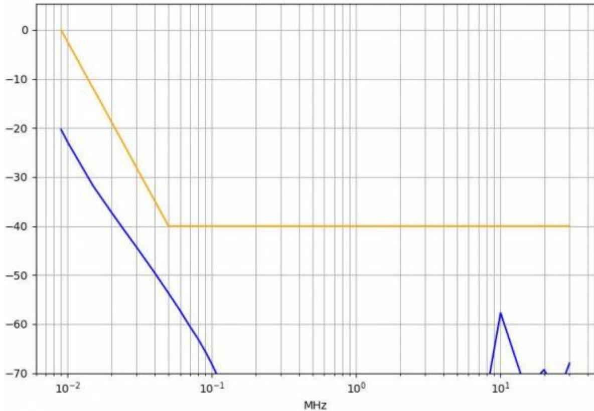
Figure 7. Isolation between mains port and RF port.
