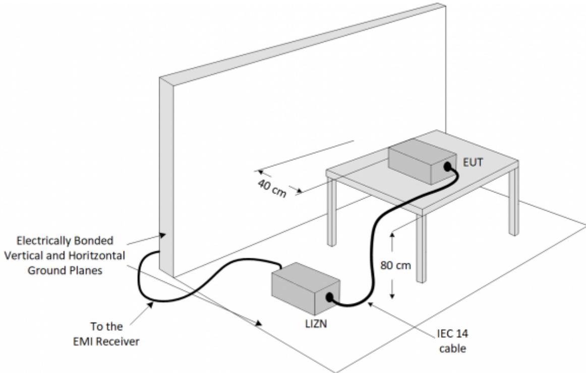
**Figure 9. Test setup for RFI voltage measurement.**
