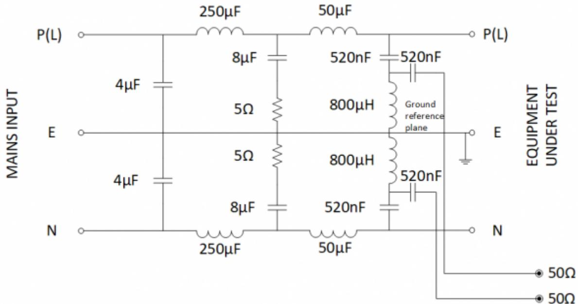
**Figure 8. Schematic of the LIZN's LISN.**
