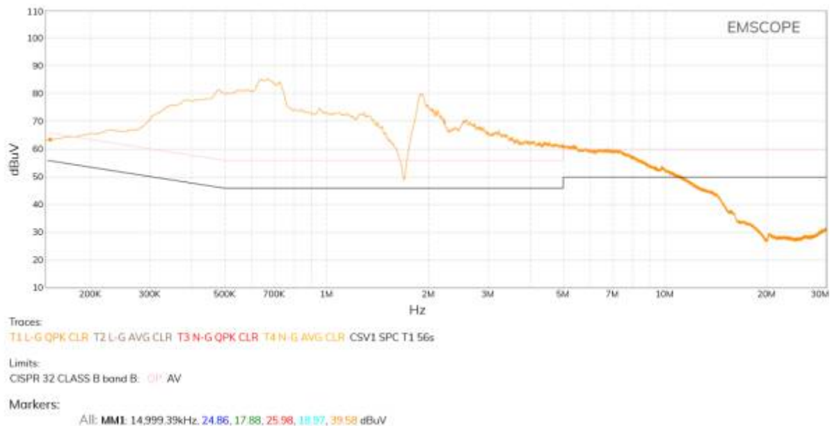
Figure 7. QPK Line emissions at a specific time slice where the cavity magnetron is on.
