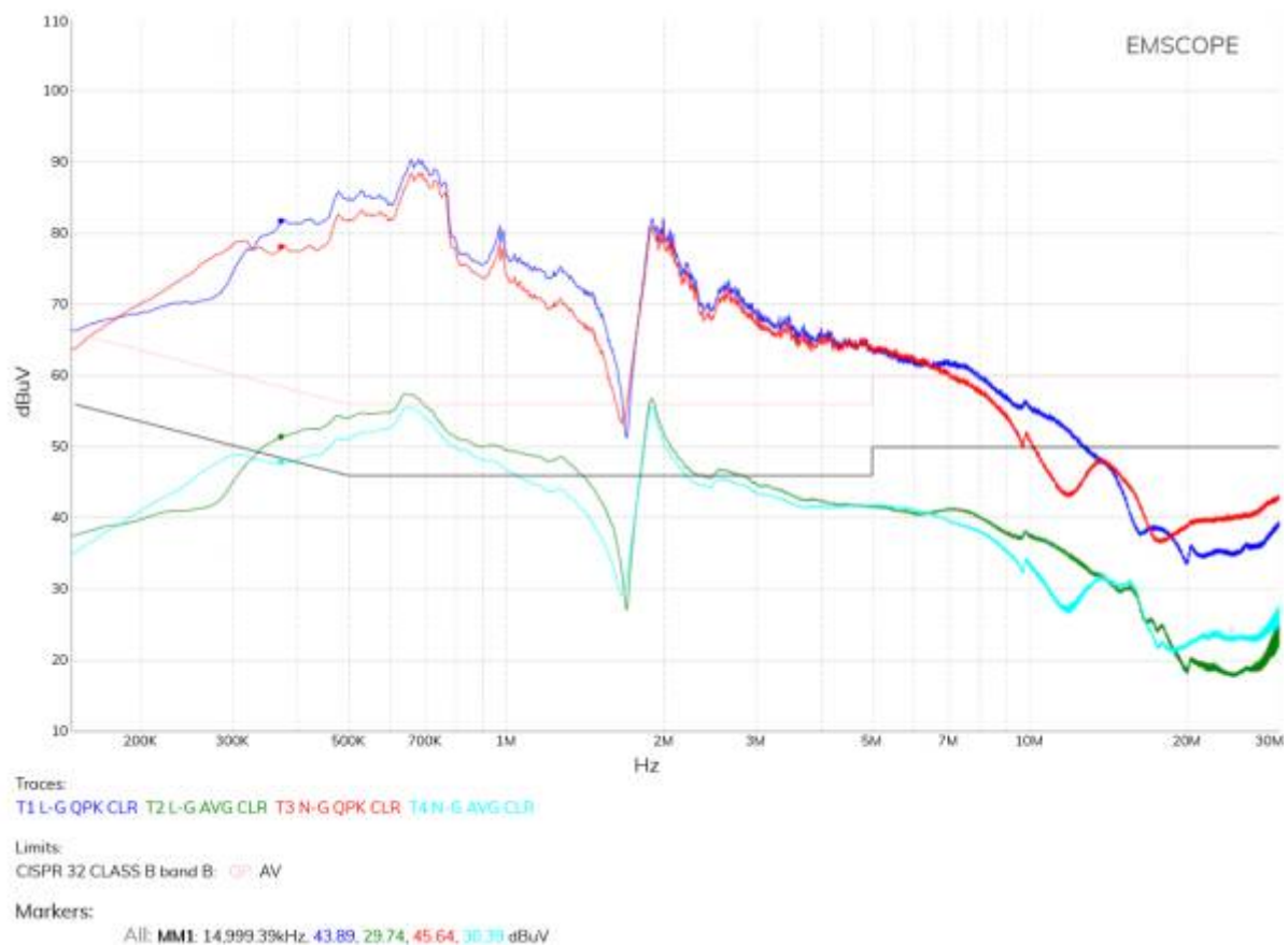
Figure 5. DUT emissions: QPK detectors: Line in blue, Neutral in red. CAVG detectors: Line in green, Neutral in cyan.
