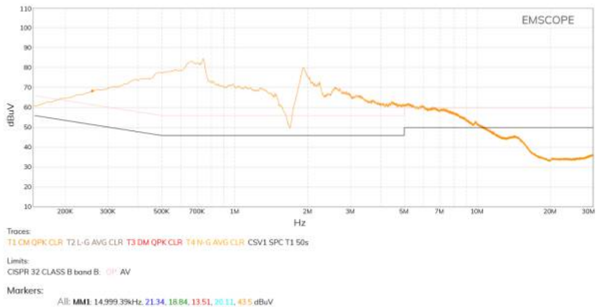
Figure 10. Common mode emissions at a specific time slice where the cavity magnetron is on. QPK detector.
